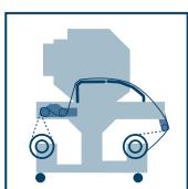
**The feeding system: winder and unwinder** JP2 operates by feeding system with rolls up to 100 Kg, assuring fast and constant paper feeding, peculiar in the industrial production.
